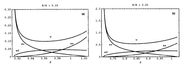
Fig. 2. The relationships  $e_s$ ,  $e_d$ ,  $e_w$  and w vs. F. Here,  $F = 1 + \epsilon \lambda$  is the Froude number,  $\epsilon = (R/H)^{1/2}$  the small number for the asymptotic analysis and R the radius of the semi-circular bump: (a) R/H = 0.1 in the interval  $(F_L, F_0) = (0.91460, 1.02407)$ , and (b) R/H = 0.25 in the interval  $(F_L, F_0) = (0.71000, 1.02410)$ .
