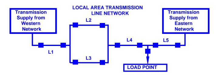
Figure 7 Partial transmission network serving a single load point.
