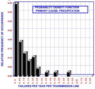
Fig 3. Relative frequency of transmission line outages - Primary cause precipitation
