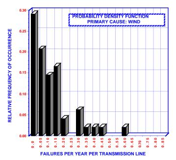
Fig 4. Relative frequency of transmission line outages - Primary cause wind
