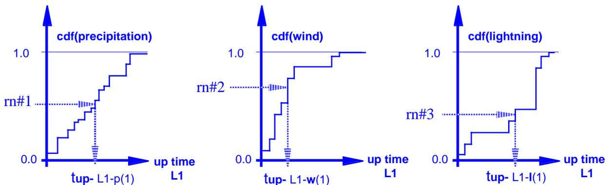
Figure 7 Cumulative distribution of adverse weather up or operational time for transmission line #1
