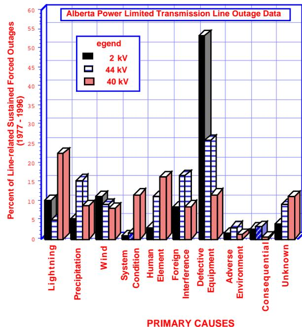
Fig 1. Primary causes of transmission line outage
