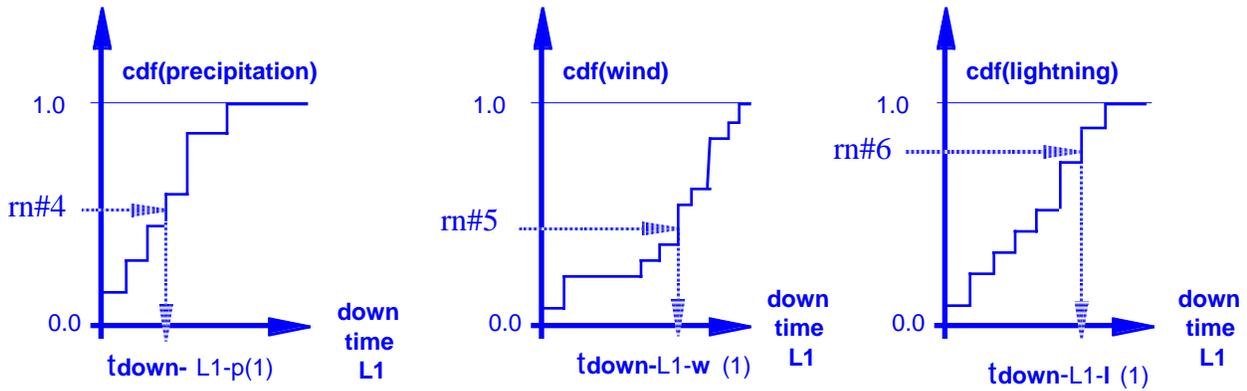
Figure 8 Cumulative distribution of adverse weather variables down time for transmission line #1
