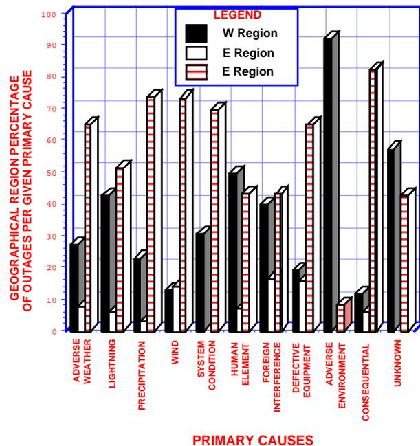
Fig 6. Percentage of transmission line outages by geographical region for a given primary cause
