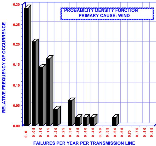
Fig 4. Relative frequency of transmission line outages - Primary cause wind
