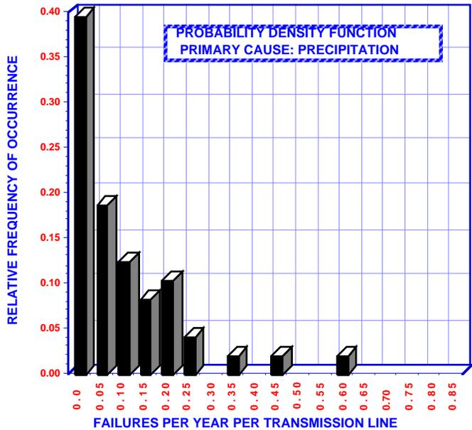
Fig 3. Relative frequency of transmission line outages - Primary cause precipitation
