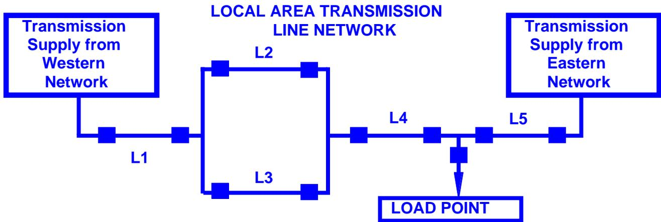
Figure 7 Partial transmission network serving a single load point.
