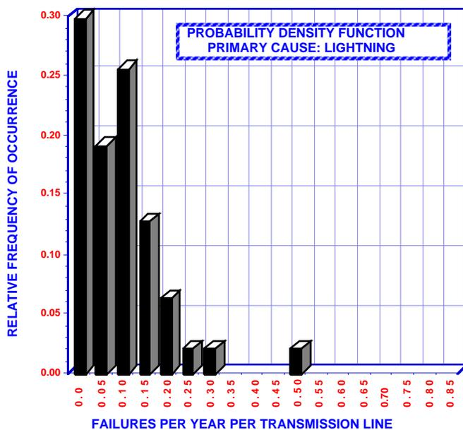
Fig 5. Relative frequency of transmission line outages - Primary cause lightning
