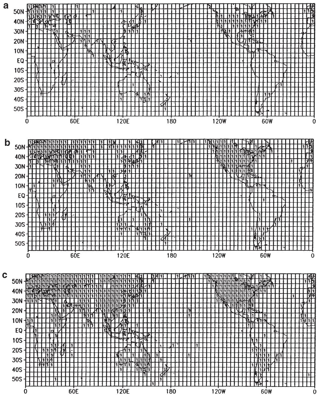
Figure 1. Representation of the global coverage of the GHCN data boxes: (a) January 1880, (b) January 1930 and (c) January 1983. The boxes with '1' indicate the existence of observed data for the month
